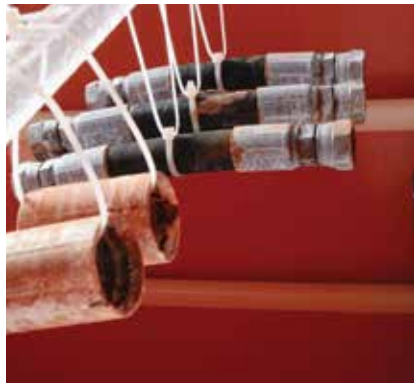
Salt spray test
