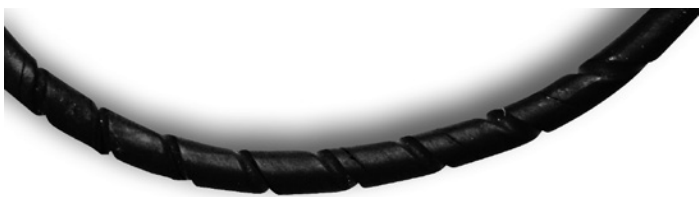
Fig. 10.9 Twisted O-ring with spiral markings
