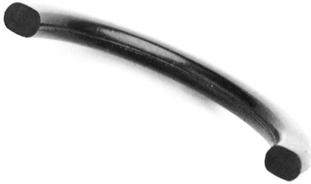
Fig. 10.8 Damage pattern caused by high compression set
